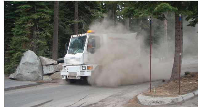
Many of the street sweepers used in Tahoe are not the best available technology for picking up fine particles that are so damaging to lake clarity.
